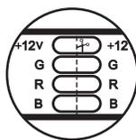
The **Underglow™** LED strips can only be cut along the leads. A 'Scissor Clipping Mark' is placed on every LED strip, designating where to cut.
